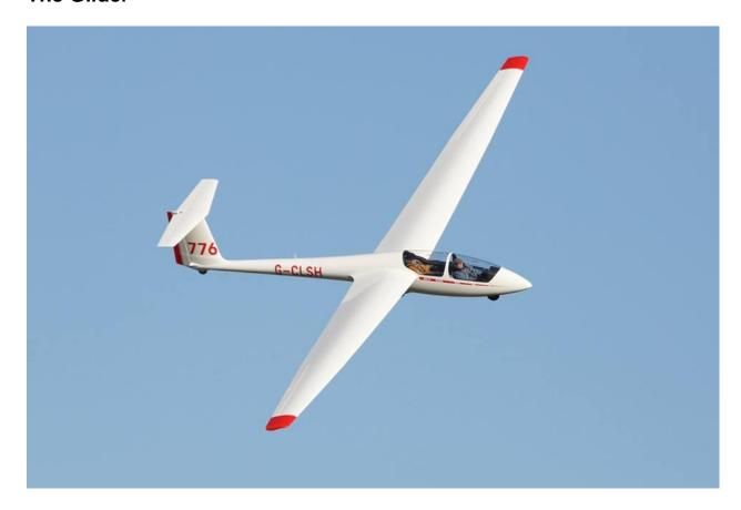
The ASK 21 is a two-seater mid-wing with 17m span, designed by Rudolf Kaiser. It is widely used in gliding clubs for basic to advanced instruction. <a href="https://www.alexander-schleicher.de/en/flugzeuge/ask-21/">https://www.alexander-schleicher.de/en/flugzeuge/ask-21/</a>
