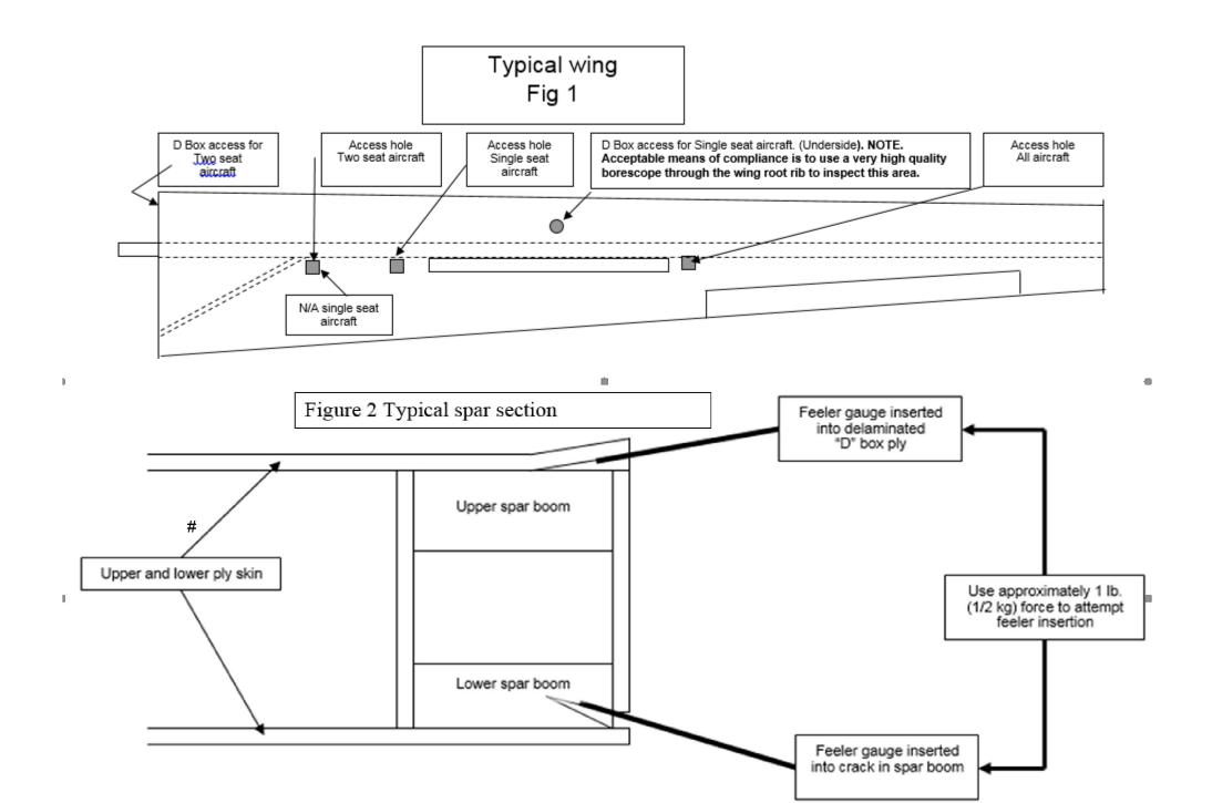
Through the inspection holes, inspect the internal structure of the wing trailing edge using a torch and mirror or suitable inspection equipment. Pay particular attention to the air brake box and drag spar attachment to the main spar.
