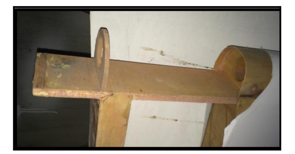
Figure 4 Typical Sternpost and base rib glue failure
