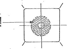
If the washer with 18 mm outside diameter is visible you can reassemble the control lever. Use a new self locking nut M 6 DIN 985.
