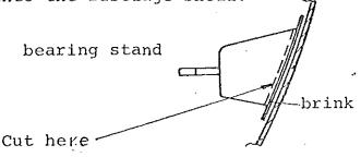
3. Abrade the brink of the bearingstand until the fiberglass of the brink is completely removed.
