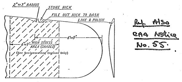
It was also stated that "a small nick at the point of peak stress may be as detrimental from the fatigue standpoint as a large nick. A quick inspection for cracks at the critical area should be included in the pre-flight inspection".
