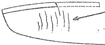
such cracks may also appear in inner blade sections.
