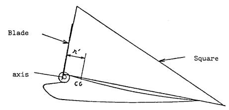
Then measure the distance r' between that blade and the marked small circle centre which is the centre of gravity and substract 3mm for the axis radius -> r. The maxi permissible miscalculation is 0,5mm. The product of the aileron weight (Kg) by the resulted length r ( in cm) give the balance which must take place inside the definite limits as shown in Service Guide : 2,8 to 3,5 cm/Kg.
