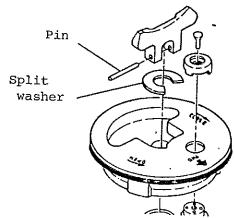
It appears from the Cessna Parts Catalogue that the pin used in the plastic caps has a different part number from the pin used in the metal caps.
