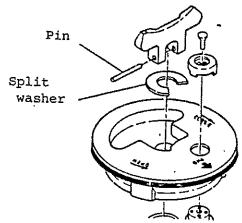
It appears from the Cessna Parts Catalogue that the pin used in the plastic caps has a different part number from the pin used in the metal caps.
