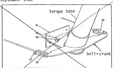
During inspection of the rudder torque tube in accordance with CAA AD 001-02-85 and the Gulfstream American Service Bulletin No ME-21, three longitudinal cracks were found in the torque tube beneath the bell crank. The 1979 aircraft has flown a total of 1150 hours.
