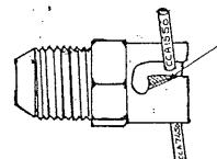
Carefully file off shaded area of slot sufficiently to prevent the valve locking in the OPEN POSITION. Vendor part number CCA 1550 (Piper P/N 492-022) and CCA 7450 (Piper P/N 492-100).
