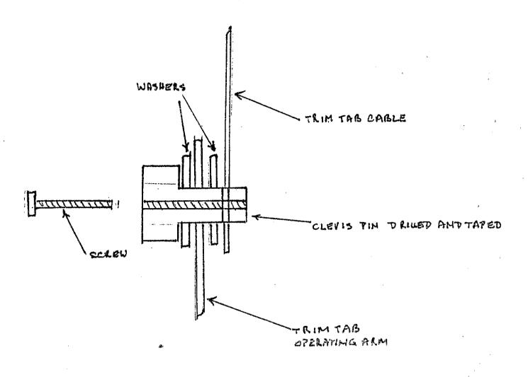
THE CLEVIS PIN IS FREE TO ROTATE IN THE TRIM TAB OPERATING LEVER. THE TRIM TAB CABLE IS CLAMPEDBY THE SCREW PASSING THROUGH THE CLEVIS PIN
