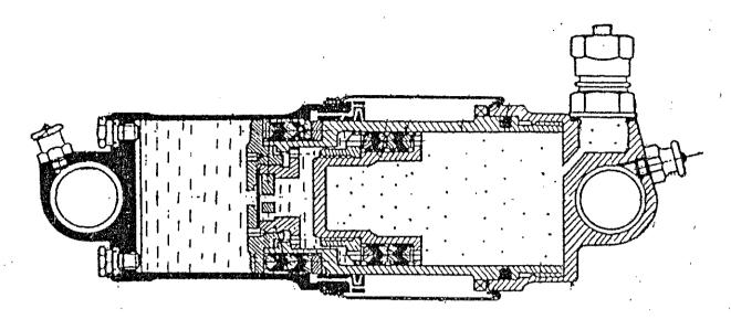
To allow the use of standard "O" rings instead of imported metric lipped seals, a modification has been developed by a Blanik operator involving the manufacture of a new piston and cap both machined to accept standard "O" rings.
