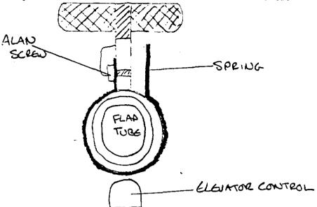
The elevator control should be checked for full movement with the flap lever in full negative position and full positive position before every flight.
