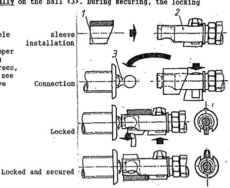
Warning: With connectors unsecured, the locking plate may open under load temporarily! The locking plate should never be greased!
