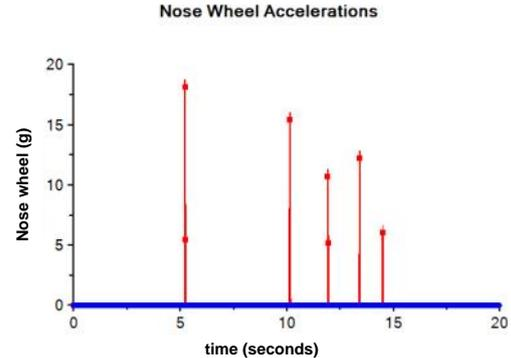
*This chart shows the series of short duration decelerations (measured in gs) calculated to be inflicted on a K13 airframe and then its occupants by the nose-wheel impacting a hard runway when the glider fails to round out and the instructor does not succeed in intervening. The decelerations shown are measured vertically.
