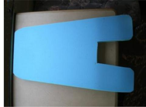
*This energy-absorbing foam insert was designed to also support the area under the pilot's thighs. This also prevented discomfort from being generated in those areas. Note that the foam inserts are always placed within a protective cloth cover to prevent them being damaged when in use.*
