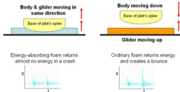
*Recognised energy-absorbing foams return almost no energy in a crash. Ordinary foams and many other materials do the opposite. The returned energy separates the pilot's bottom from the seat. This means the pilot can end up descending and meeting the glider structure coming the other way as it, in turn, bounces off the ground. The gs experienced in such circumstances might be greater than the initial impact. This is illustrated in the graphs in the figure.*
