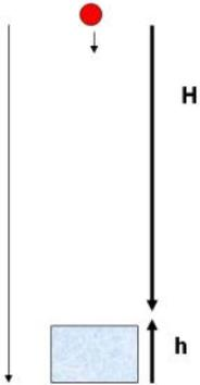
*This shows an object free-falling for a distance  $H$  and then being decelerated uniformly to rest in distance  $h$ .*
