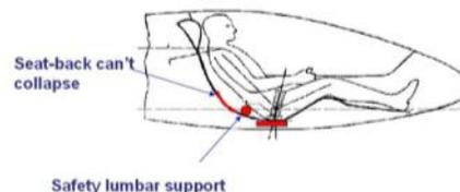
*Other precautions, which count as personal removable equipment, are a lumbar support made out of a recognised energy-absorbing foam and a removable insert made out of the same material to place in any large void behind the seat back. Under the overwhelming forces that can be involved in a crash, these measures should help stop the lower spine being bent and forced into the space that would otherwise exist.*
