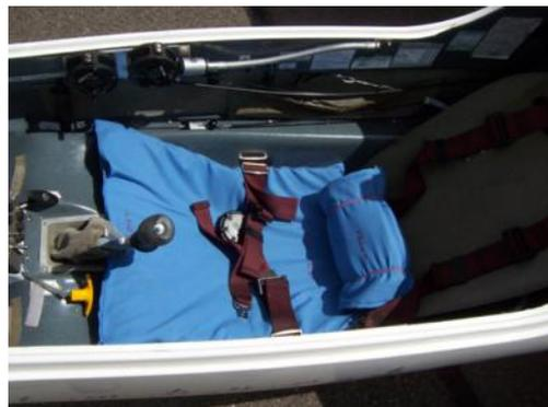
*This shows a lumbar support on the right-hand side made out of energy-absorbing foam sitting on top of the back of a fitted energy-absorbing safety cushion.*
