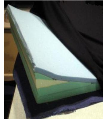
*This shows the energy-absorbing foam layers used in the make-up of a particular safety lumbar support. It is important that such a support is not oversized so that it generates discomfort. The lower back should rest comfortably on this during flight so that, in the event of a crash, the lower back immediately starts to decelerate with the aircraft as opposed to first passing through a void and bending significantly in the process.*
