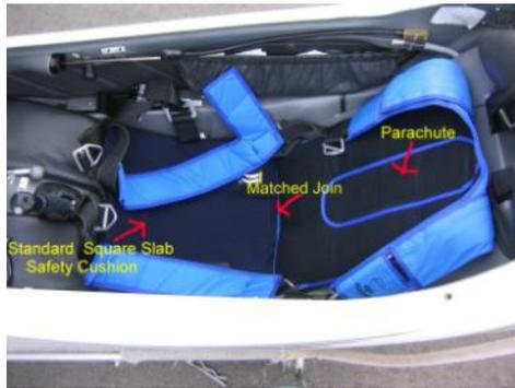
*This shows a standard square safety cushion installed alongside a parachute. The thickness of the safety cushion matches the base of the parachute. This has minimised any void and consequent lack of support in the lumbar region.*
