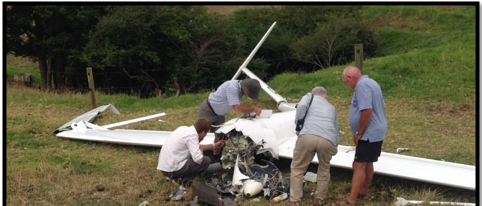
Caused by incorrectly fitted parcel shelf during maintenance
