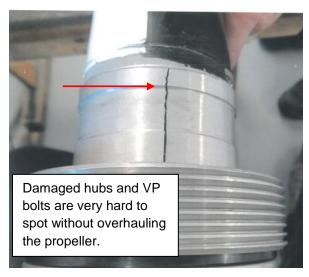
Cracked prop hub, caused by expanding wooden/composite blade. This prop was less than 5 years old when damage found due to small expansion cracks in prop blade.
