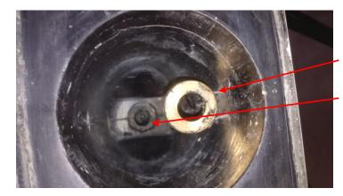
Loose wing tip spigot bush in wing (in this picture it is totally detached) This results in the tip being a very loose fit. (check play every rig?)
