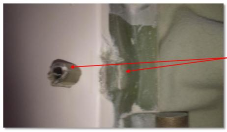
Broken aileron hinge only found when Mylar removed.
