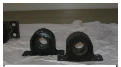
These are rubber LS4 undercarriage mounts. They have a limited life. No perishing or bulging allowed. When buying new mounts, inspect carefully before fitting them, as they have often sat on a shelf for many years and are unacceptably perished.
