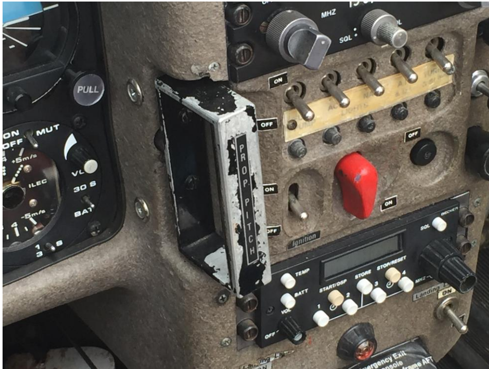
Fig 6. Propeller pitch change handle and adjacent ignition switch
