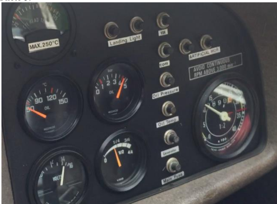
Photo 5. Engine idling at 1100 rpm with the throttle closed.
