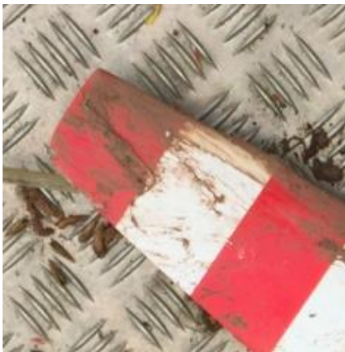
Photo 3. Propeller tip area. Note the absence circumferential scoring/LE damage.
