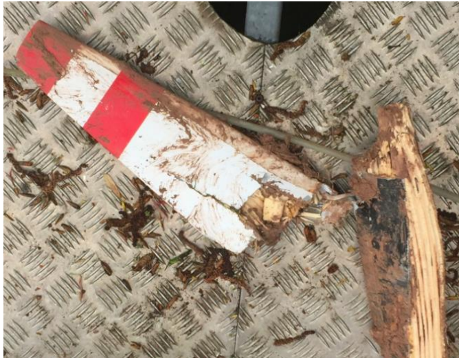
Photo 2. Broken, not shattered, propeller blade
