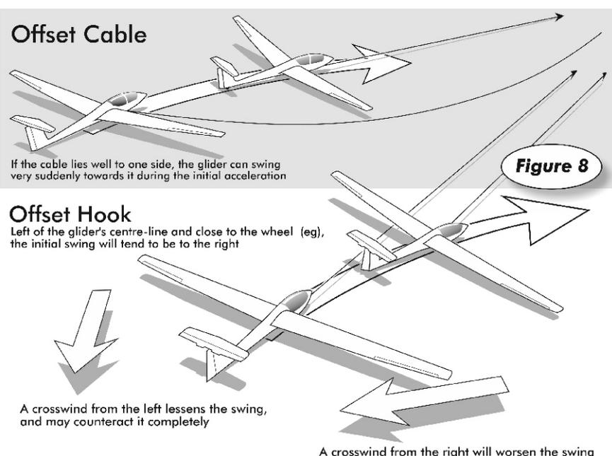
It's easy to get into the habit of being slightly out of line, always just far enough to make miles out of line seem OK, which it is not. Sites which use retrieve winches may seem to be launching with the cable's pull far more out of line than is actually the case. The geometry of these set-ups is such that by the time the glider starts to move the cable pull has become more or less in line with the glider's fuselage. Nevertheless, the accident described is not impossible at such sites.
