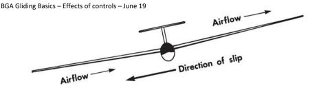
In consequence the lower wing meets the sideways component of the airflow at a greater angle of attack than the upper wing and will therefore have more lift. This greater lift restores the aircraft to the normal level position.
