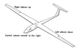
Movement of the stick to the left raises the left aileron and depresses the right aileron. Thus, the left aileron presents a reduced angle of attack to the airflow, and therefore gives less lift; the right aileron, having been lowered, presents an increased angle of attack and hence gives more lift.
