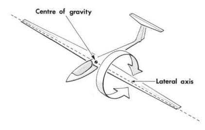
**Remember** - No matter what the attitude of the aircraft is in relation to the ground, the controls always have the same primary effect on the aircraft (unless it is stalled). The ailerons give control in the rolling plane, the elevator in the pitching plane and the rudder in the yawing plane. These planes are referred to the aircraft and not to the earth.
