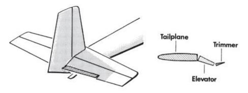
The trimmer is used to relieve the pilot of work in maintaining the required attitude in pitch. If, for instance, the pilot wishes to fly faster, she moves the stick to effect the necessary change of attitude and then, once the speed is steady, adjusts the trim until the aircraft maintains that attitude without any need for pressure on the stick. Remember set the *attitude*, check correct *speed* and then adjust the *trimmer*.
