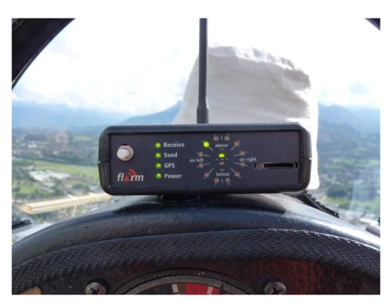
FLARM showing another FLARM equipped aircraft on a potential collision course. The FLARM unit is indicating that the other aircraft is left of the nose and higher.
