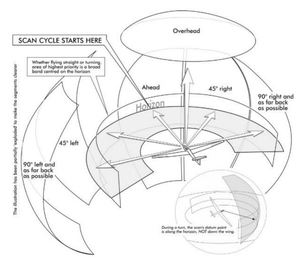
The scan pattern described is an idealised one and should be regarded as an elastic framework rather than a pattern to be rigidly adhered too. The first and most important point is to have a scan pattern that covers everything that needs to be covered. The second point is that the pattern should become so ingrained that you will continue to look out even when tired, which is one occasion when it tends to get forgotten.
