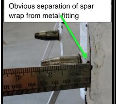
But the other side of the spar wraps has previously been cut away to treat corrosion! The wrap should have been replaced
