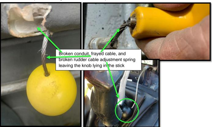
This is not an easy spot. There is not much space in the air brake box (note, some later Puchacz's have a different end fitting). Inspect thoroughly at next maintenance and report to the BGA if any problems found.
