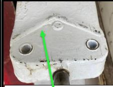
Another wing that has had the spar wrap cut away to treat corrosion, and not replaced.
