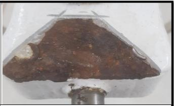
This amount of corrosion requires the removal of the metal fitting and very likely replacement. Now removed, the fitting might need to be replaced. Contact Streifly about the rivets.
