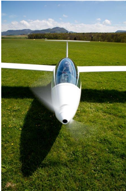
Discus FES, 22 kW engine (but will fly on 4kW)
