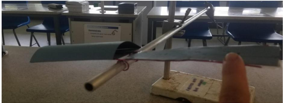
11. This can now be mounted on a clamped metal rod so the wing can pivot around the centre loops of copper (Figure 6). The wing should be unbalanced with the platform pointing upwards
