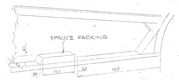
3. Cut away inner skin in cockpit to admit packing 50 x 20 x 13 and canopy catch locking bracket. Drill through longeron for 2 BA Bolts. (See below)
