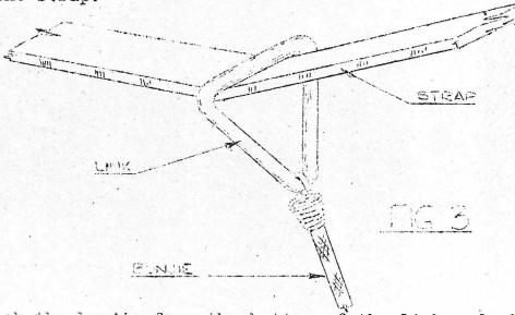
6. Attach the bunjie from the bottom of the link ref: SK42/100/200/D to the plate Ref: SK42/100/200/F in the starboard side of the canopy, as in fig 3. Attach the eheck strap to the plate Ref: SK 42/100/200/E on the port side of the canopy. This completes the embodiment of the modification.
