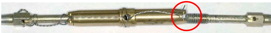
Fig. 1 Picture of the failed Turnbuckle: As shown in the red circle, the safety wire was cut by the groove originally designed to accommodate a locking clip. As a result, the flight control cable end at the right of the picture unscrewed and eventually got loose
